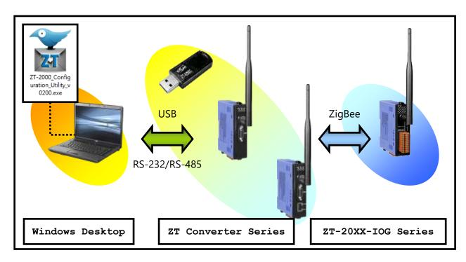
(2) For building the wireless communication of the ZT-20xx-IOG and the ZigBee converter, first, set up the following parameters of the ZigBee converter via the "ZT-2000 Configuration Utility", so it can wirelessly communicate with the ZT-20xx-IOG that in the INIT mode.
