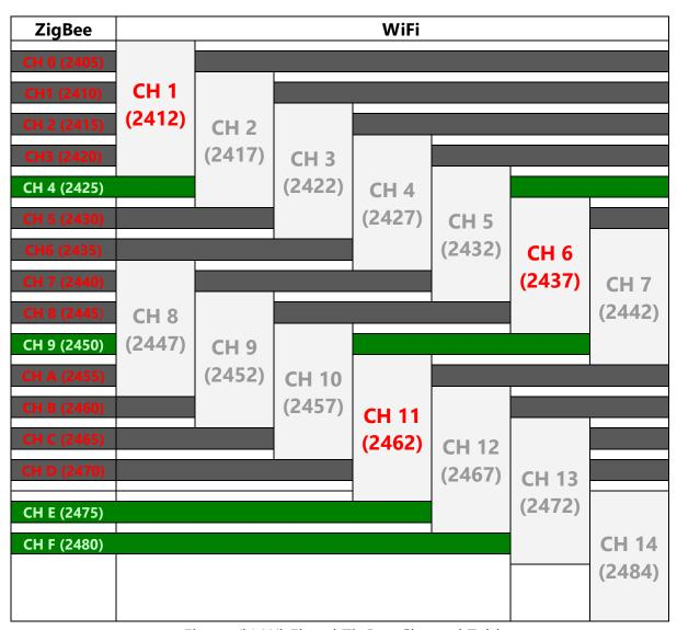
Figure (b) Wi-Fi and ZigBee Channel Table
