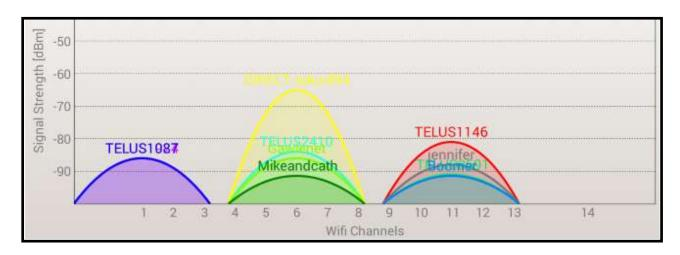
Then, from the following 【Figure (a) Wi-Fi and ZigBee Channel Diagram 】, the frequencies of the using Wi-Fi channel 1, 6 and 11 are 2412±11 (MHz), 2437±11 (MHz) and 2462±11 (MHz). These 3 channel ranges are the radio interference source for the ZigBee network in the same band; So, the better ZigBee options that recommended in this case are 2423 ~ 2426 (MHz), 2448 ~ 2451 (MHz) and 2473 ~ 2480 (MHz).
