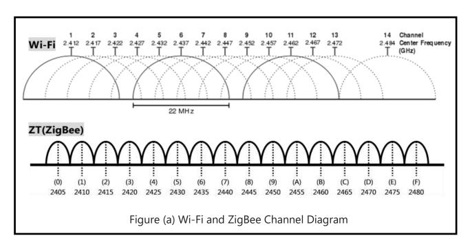
Then, from the 【Figure (b) Wi-Fi and ZigBee Channel Table】, we know the three ranges 2423 ~ 2426 (MHz), 2448 ~ 2451 (MHz) and 2473 ~ 2480 (MHz) are the ZigBee channels 4, 9, E and F, so these four ZigBee channels may be preferred selecting to avoid overlap with the WLAN.
