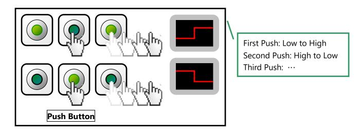
(3) The emergency bell alarm system for the toilet in campus, to avoid the emergency messages being maliciously released, can use the "Emergency Button" as an alarm trigger that has the difficult to reset feature.
