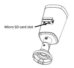
**NOTE:** Do not hot plug the memory card after it has been inserted and the power turned on, otherwise, the camera or the card might be damaged.
