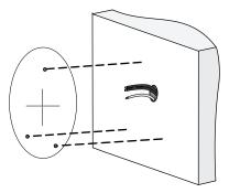
3. Drill the screw holes. Depending on the material of the surface where the camera will be installed, it may be necessary to drill the three (3) screw holes and use the supplied screw tox.
