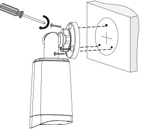
3. Adjust the camera tilt angle, then fasten the head screw to fix the camera angle position.
