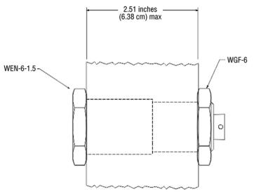
WGF-6-1.5 attached to WGF-6 installed in SCIF wall
