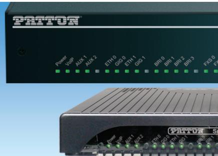
The SN5550 is a cost effective eSBC with integrated Broadband access and a variety of telephony port combinations of BRI/FXS/FXO. It is capable of doing up to 200 SIP to SIP calls\*\*\* whereof max. 8 can be transcoded\*\*. Built-in QoS functionalities and support of G.722 high definition codec, ensure excellent VoIP call quality.
