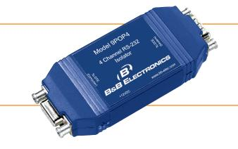
The 9POP4 isolates and protects RS-232 equipment from lightning surges, accidental high voltage shorts, and ground loops. RS-232 data signals TD, RD, RTS, and CTS are supported at up to 230.4 kbps. Isolation circuits are 2.5 kV rated and protects valuable equipment while maintaining maximum uptime.
