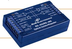
Model 4850P is an optically isolated RS-422/485 signal repeater. In addition to 2KV isolation on the data lines, it can be used to extend RS-422/485 circuits an additional 1.2 km (4,000 ft.), thereby doubling the range. An added benefit is the ability to add another 32 nodes to an RS-485 network and join 2 and 4 wire systems.
