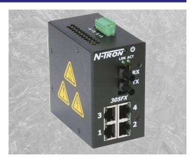
The 305FX can simplify plant wiring by eliminating the need to bring data acquisition and control network connections back to a climate controlled environment. The 305FX has extended operating environmental specifications to meet the harsh needs of the industrial environment. For cost savings and convenience the 305FX can be DIN-Rail mounted alongside Ethernet I/O or other industrial equipment.
