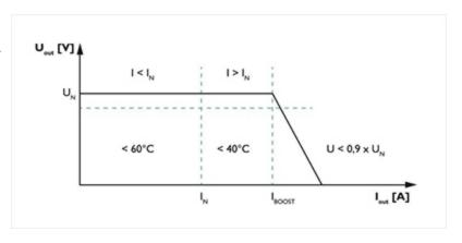
capacitive loads have to be absorbed without voltage dips. With the QUINT Power Boost function a static boost will continuously provide up to 125% of the nominal current. In addition, you can use the dynamic boost to supply 150% of the nominal current for 5 seconds when starting up heavy loads.
