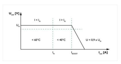
capacitive loads have to be absorbed without voltage dips. With the QUINT Power Boost function a static boost will continuously provide up to 125% of the nominal current. In addition, you can use the dynamic boost to supply 200% of the nominal current for 5 seconds when starting up heavy loads.
