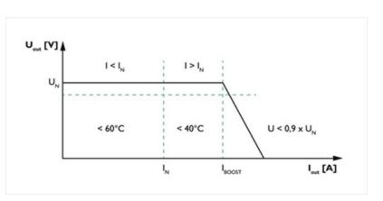
switch-on currents of capacitive loads have to be absorbed without voltage dips. With the QUINT Power Boost function a static boost will continuously provide up to 125% of the nominal current. In addition, you can use the dynamic boost to supply 200% of the nominal current for 5 seconds when starting up heavy loads.
