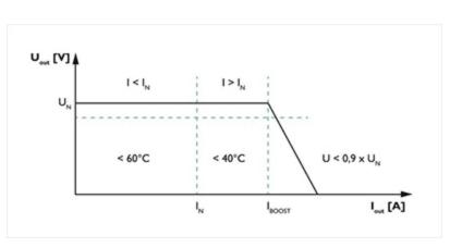
capacitive loads have to be absorbed without voltage dips. With this QUINT Power Boost function a static boost will continuously provide up to 125% of the nominal current.
