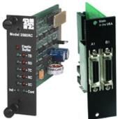
The Model 2021 is typically used in LAN-WAN connectivity, video conferencing and other high speed applications where one vendor's DCE is required to communicate with another vendor's DTE.
