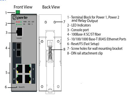
Note: Fiber Port may appear different, depending on the type of fiber port installed.
