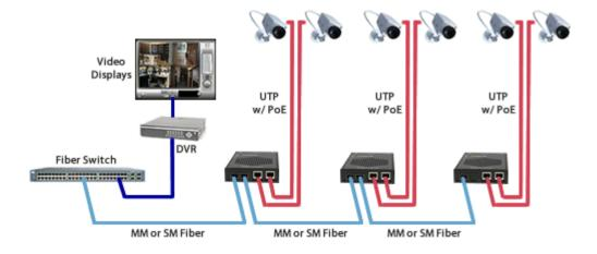
A second option is to have redundant fiber links for installations requiring fiber facility protection. There is an active fiber port and a protection fiber port that can support a fiber failure switchover of less than
