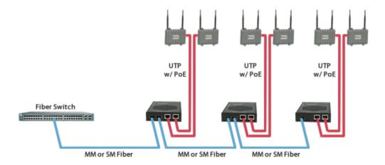
A second option is to have redundant fiber links for installations requiring fiber facility protection. There https://www.perie.com/products/media-converters/s-1100p-sip-in-poe-media-converters/shtml 50 milliseconds. The PoE+ media converter supplies power to the camera, and has power protection from an Uninterruptible Power Supply (UPS) battery back-up. In the event of a fiber cut and a loss of power, the camera continues to send data on the protection link.
