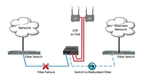
2. **Redundant Primary** : When the primary link fails, the media converter redirects traffic to the secondary fiber port within 50ms. Upon restoration of the primary fiber link, traffic is automatically redirected back to the primary fiber.
