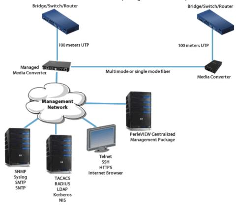
10/100 - Extend Network between Ethernet Hubs
