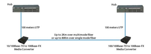
10/100 - Extend Network between 10Mbps and Fast Ethernet
