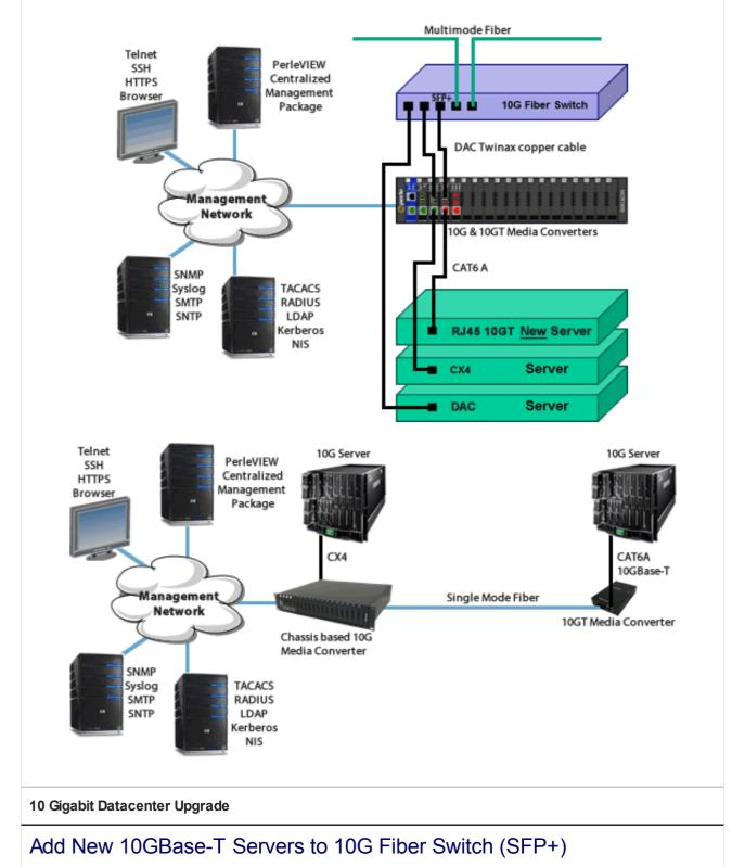
Install new 10GBase-T Servers to existing top of rack switches. Connect your 10GBase-T server to SFP+ Switch with Direct Attach DAC copper cable. 10G Media Converters can also connect CX4 servers to SFP+ Switch.
