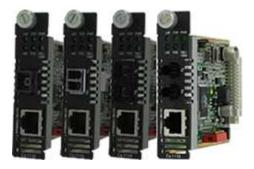
Installed in a high density Perle Media Converter Chassis, Perle's line of feature rich **Managed Gigabit Media Converter Modules** transparently connect copper to fiber. Our Gigabit Ethernet to Fiber Converters provide an economical path to extend the distance of an existing network, the life of non-fiber based equipment, or the distance between two devices.
