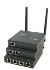
Delivering high performance in a compact size, the IOLAN SDS L offers support for a broad range of 4G LTE cellular data networks, extensive security, flexibility and IPv6 technology making it ideal for applications that require remote serial console management, data capture or monitoring.
