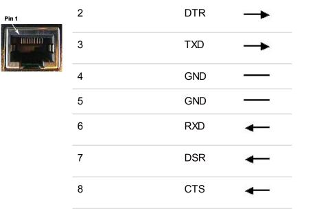
( A rolled RJ45 cable will automatically perform DTE to DCE crossover )
