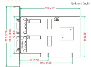
602U-I CAN interface board uses the NXP SJA1000 and transceiver PCA82C251, which provide the bus arbitration and error detection. The -40 to 85°C wide operating temperature (CP-602U-I-T only) and 2 kV isolation make the boards suitable for use in harsh industrial environments.
