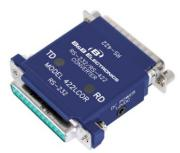
The RS-232 port uses a female DB-25 type of connector with pins 2 (TD input) and 3 (RD output) supported. Protective Ground (pin 1) and Signal Ground (pin 7) are also connected. The RS-422 port uses a male DB-25 type of connector with the Send Data outputs on pins 2 and 14, and the Receive Data inputs on pins 5 and 17. Protective Ground (pin 1) and Signal Ground (pin 7) are connected through to the RS-232 connector.
