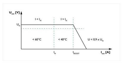
capacitive loads have to be absorbed without voltage dips. With this QUINT Power Boost function a static boost will continuously provide up to 125% of the nominal current.
